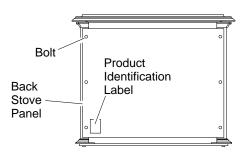
Figure 6 - Removing Back Panel
